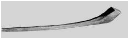
An ash wood shaft in the making. The shaft is cut in an octagonal form. The root part is not yet cut into the shape to fit into the opening in the rear end of the club head. –
